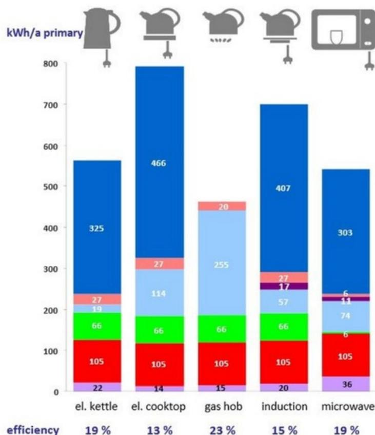
Boiling water preparation energy impact (kWh primary energy for 1,000 litre useful boiled water per year) for different cooking devices. Dark blue: power generation loss. Light blue: heat loss. Red: theoretical minimum. Pink: production, distribution, end-of-life. Pink: extra boiling time. Purple: standby. Green: over-filling. Source: "Quooker Energy Analysis", Part one, Van Holsteijn en Kemna B.V. (VHK)
