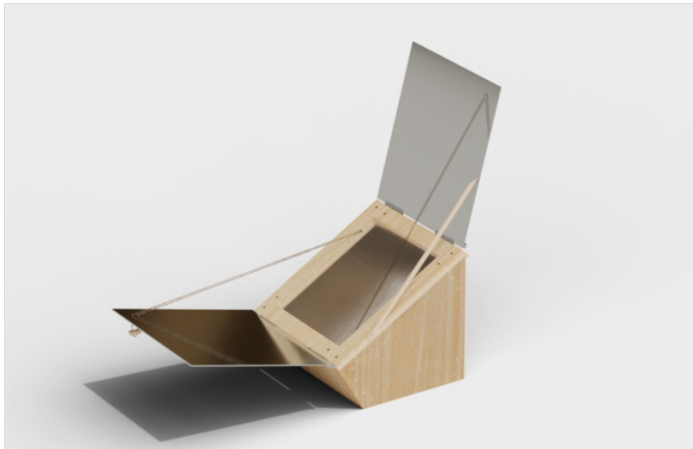
3D Model Box Solar Oven - version n°1 (based on David Mercereau design) Author: Quentin Plisson CAD Software: FreeCAD 0.20 Rendering engine: Blender / Cycles X Date: 24/07/2022
