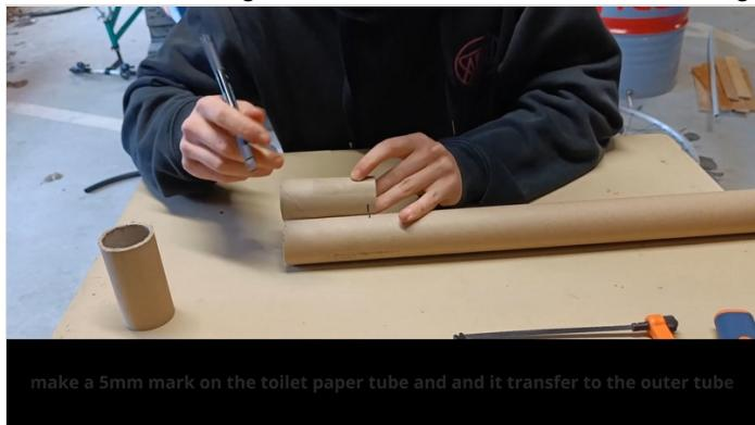
make a 5mm mark on the toilet paper tube and transfer it to the outer tube
